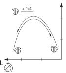
CAUTION! If the chain rotates while idling the T-screw must be turned anti-clockwise until the chain stops.
